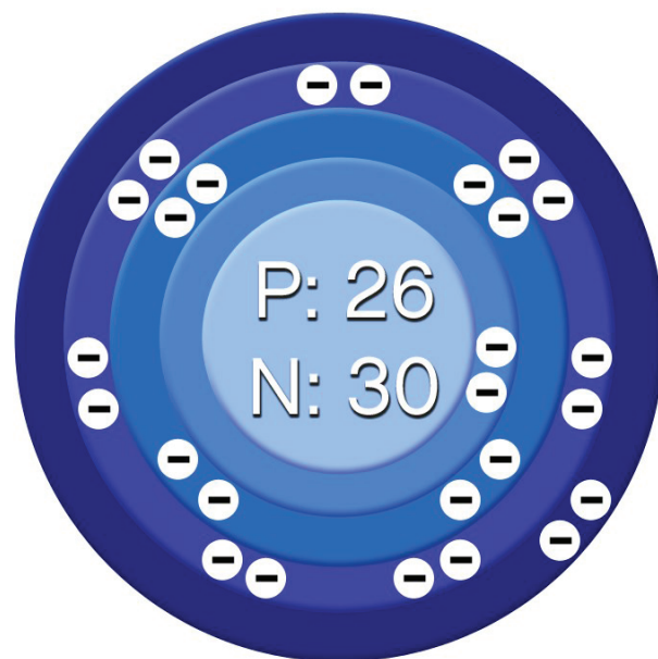
Figure 1: Atomic structure of iron.
