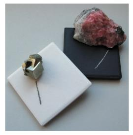
**Figure 5.** Pyrite (FeS<sub>2</sub>) (on the left) leaves a black streak, whereas rhodochrosite (MnCO<sub>3</sub>) (on the right) leaves a white streak. Photo by <u>Ra'ike</u>
