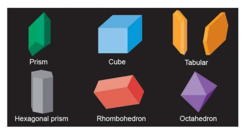
**Figure 6.** An example of some common crystal habits. The flat surfaces of these habits are known as crystal faces.
