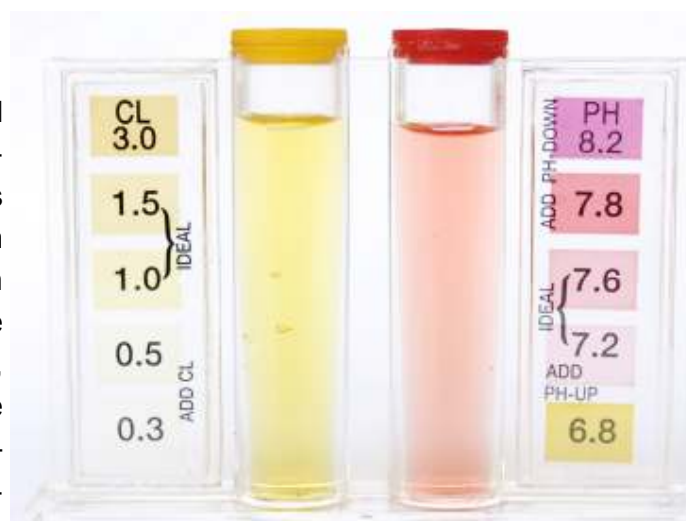
Figure 1: Swimming pool test kits are used as small titration experiments. These kits first use a phenol red indicator to measure the acidity of the pool water. Then, a titrant is slowly added drop by drop until the ideal pH is created. The number of drops added indicates how acidic the pool water was initially.
