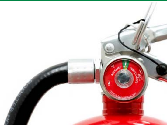
Figure 1: Pressure gauges are found wherever monitoring the pressure of a gas is important—such as this fire extinguisher above. Simple gauges are commonly used to measure the pressure of air in automobile and bicycle tires.
