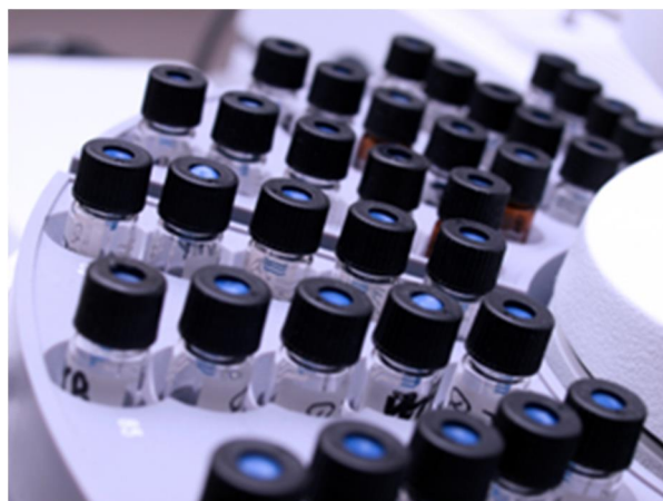
Figure 2: One type of chromatography used in laboratories is gas chromatography (GC). This is a picture of an GC autosampler.
